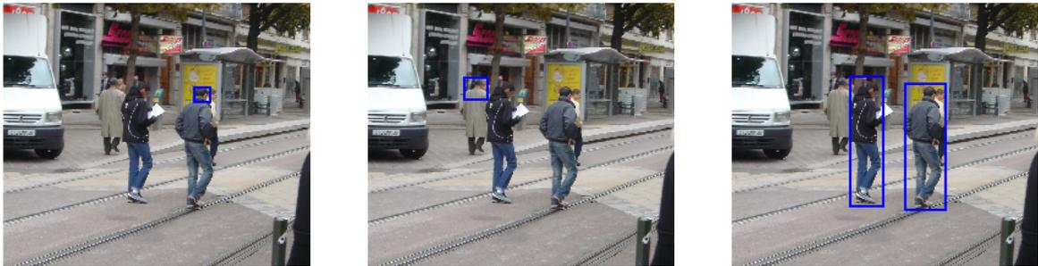
Figure 6.3: Example of inferences to the same image. The figure displays inferences of RetinaNet to *head*, *head-shoulder* and *body*, respectively. Combining the inferences would result in the correct detection of three pedestrians.
